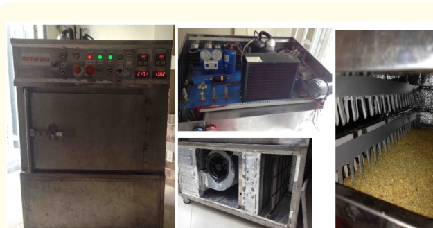
Figure 2: Installed pollen dryer on heat pump drying principal in the combination of stirring and mixing.
